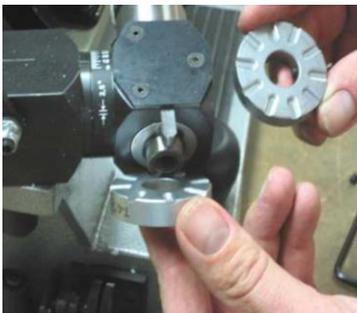
9. Tighten the index plate with the bolt, and return the index knob.
